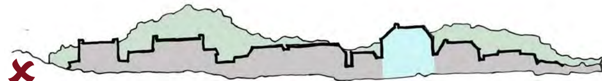
Above: New building out of scale with existing street scene
