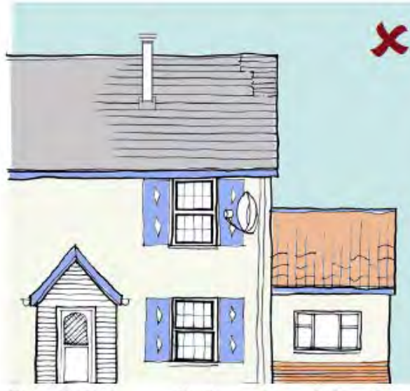
Example 2: Unsympathetic repairs and alterations
